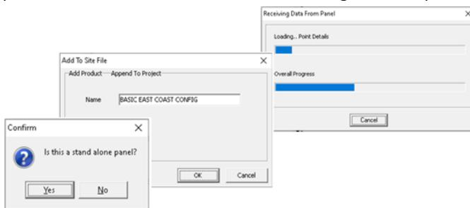
7. On completion of data transfer, save the config onto the PC
